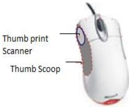
**Fig.2 Proposed biometric mouse indicating the proposed position for the thumb print scanner (for a right hand user)**
