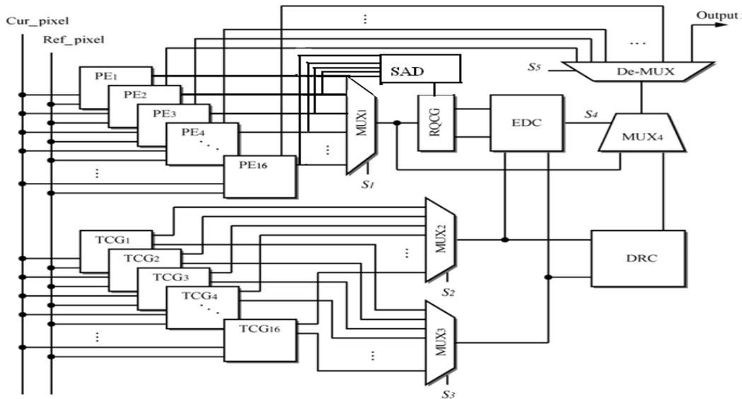
**Fig. 1. Proposed EDDR architecture design for a Motion Estimation**
