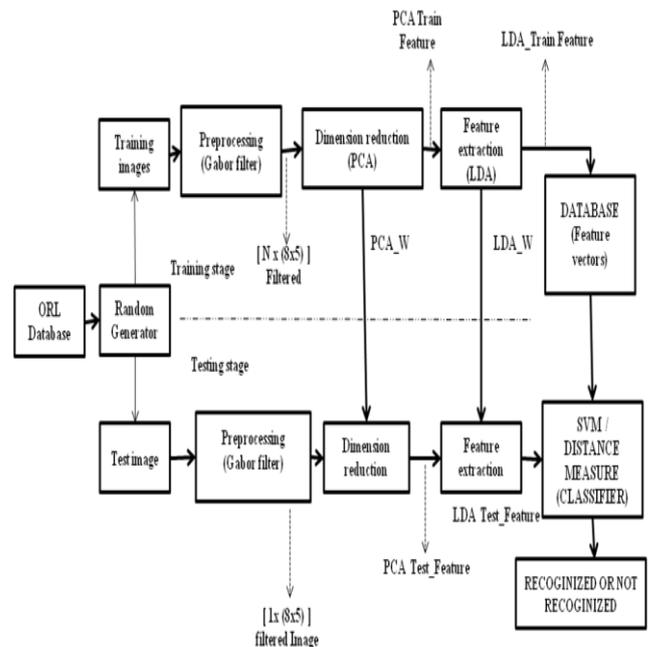
**Fig. 4. Block diagram of the proposed face recognition system**
