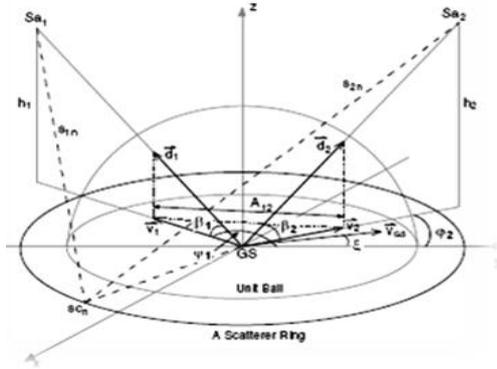
**Figure 1: the 3-D channel model for the channel between satellite Antennas and ground station antennas with the projected distance  $A_{ij}$**
