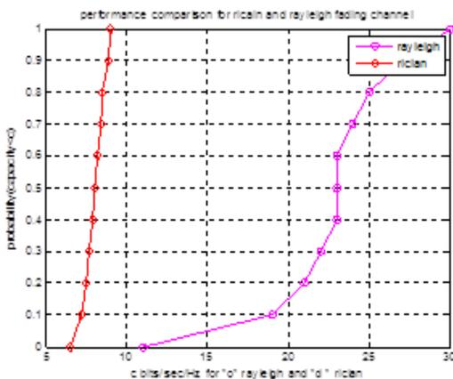
**Figure 2: comparison between rician and Rayleigh fading channel at  $d=0.5\lambda$**
