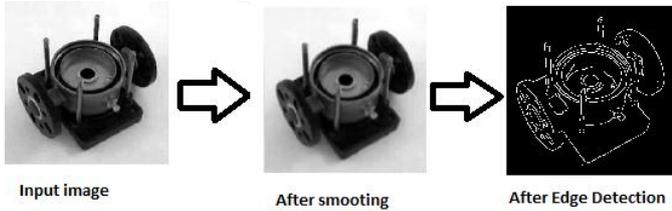
Fig 2: An image after smoothing and edge detection.
