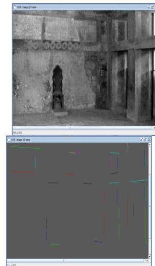
Fig 4: (a) Gaussian smoothing, (b) Canny edge detection
