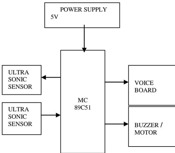
**Fig.4 ultrasonic sensor with microcontroller**
