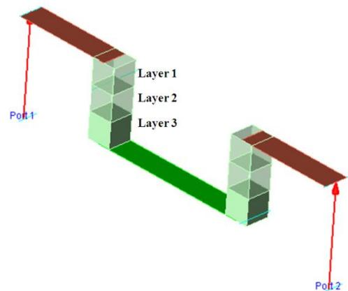
**Figure 3: PCB layer with Via**
