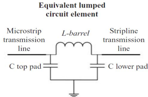
**Figure 2: Lumped model of Via**
