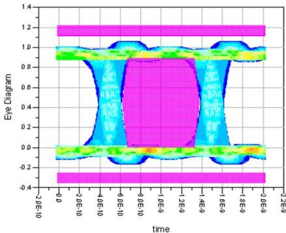
**Figure 5: Eye Pattern after via placement**
