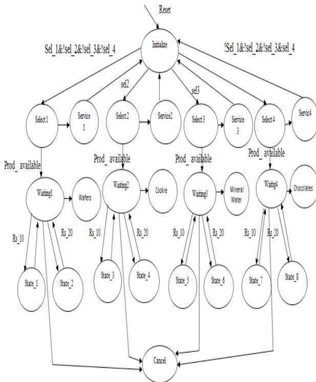
Figure 4: Finite State Machine Diagram of Vending Machine
