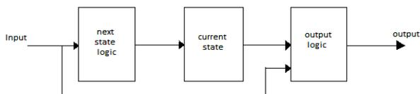
Figure 1. MEALY Machine Model.
