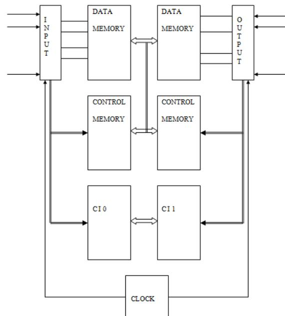
Fig 4. The Landline Switching architecture
