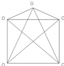
Fig 1. A network with point to point connection
