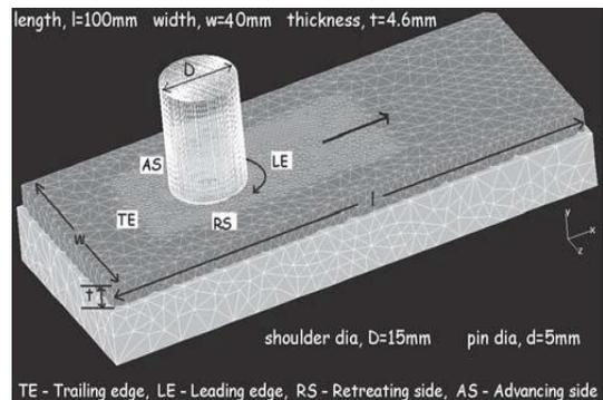
Figure 5. Setup of FSW for numerical simulations [8]
