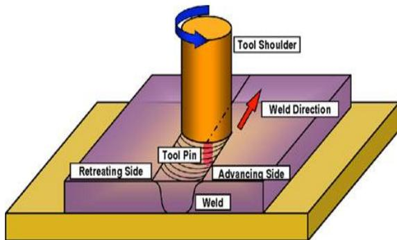
Figure 1. Process of friction stir welding [13]
