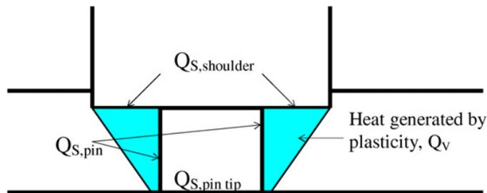
Figure 3. Schematic of the heat generation by friction at the tool/workpiece interface and by plastic deformation in the TMAZ [2]
