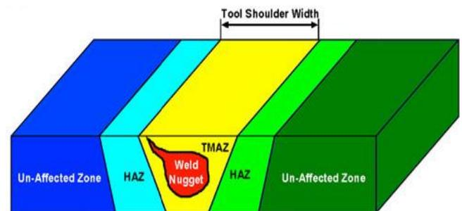
Figure 2. Various microstructural areas in FSW welds [13]
