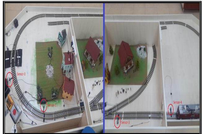
**Fig. 5. View of vibration sensors on the right side of the system**
