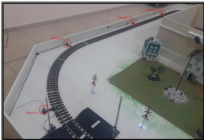
**Fig. 9. View of vibration sensors on the left side of the system**
