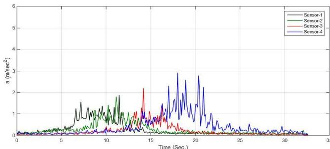
**Fig. 10. Acceleration variation train system with 0,35 m/sec speed for left side**
