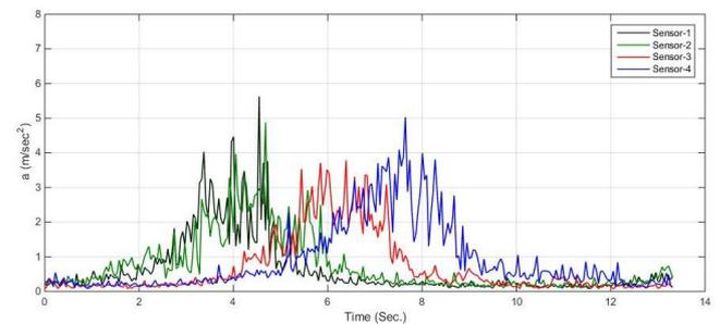
**Fig. 12. Acceleration variation train system with 0,95 m/sec speed for left side**
