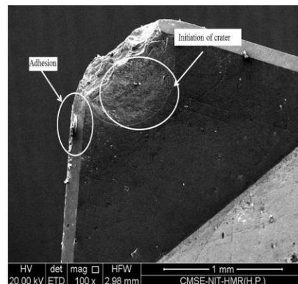
**Fig. 7** Continuous machining at 102 m/min and 20 passes
