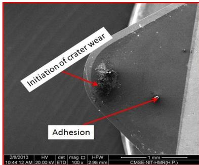
**Fig. 4** Interrupt machining at 102 m/min and 20 passes
