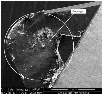
**Fig. 5** Interrupt machining at 60 m/min and 10 passes
