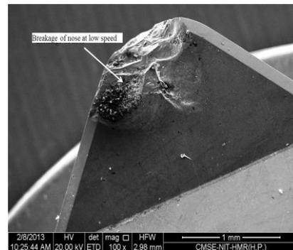
**Fig. 6** Continuous machining at 60m/min and 15 passes
