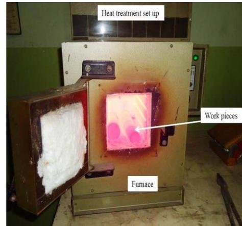
**Fig. 3 Heat treatment set-up for hardening and tempering**
