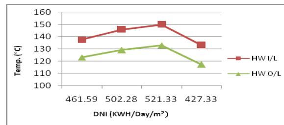
**Fig. 4 Performance graph of DNI vs Hot Water Temperature**
