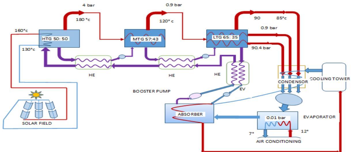
**Fig. 2. Schematic diagram of the solar vapour absorption cooling system installed**
