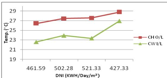
**Fig. 6 Performance graph of DNI vs Cooling water Temperature**
