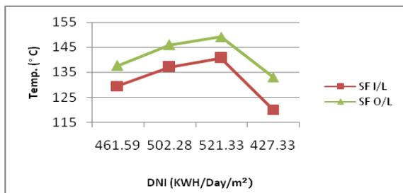
**Fig. 8 Performance graph of DNI vs Solar Field temperature.**
