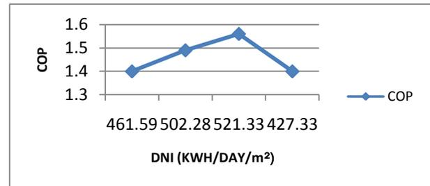
**Fig. 13 Performance graph of DNI and coefficient of performance**
