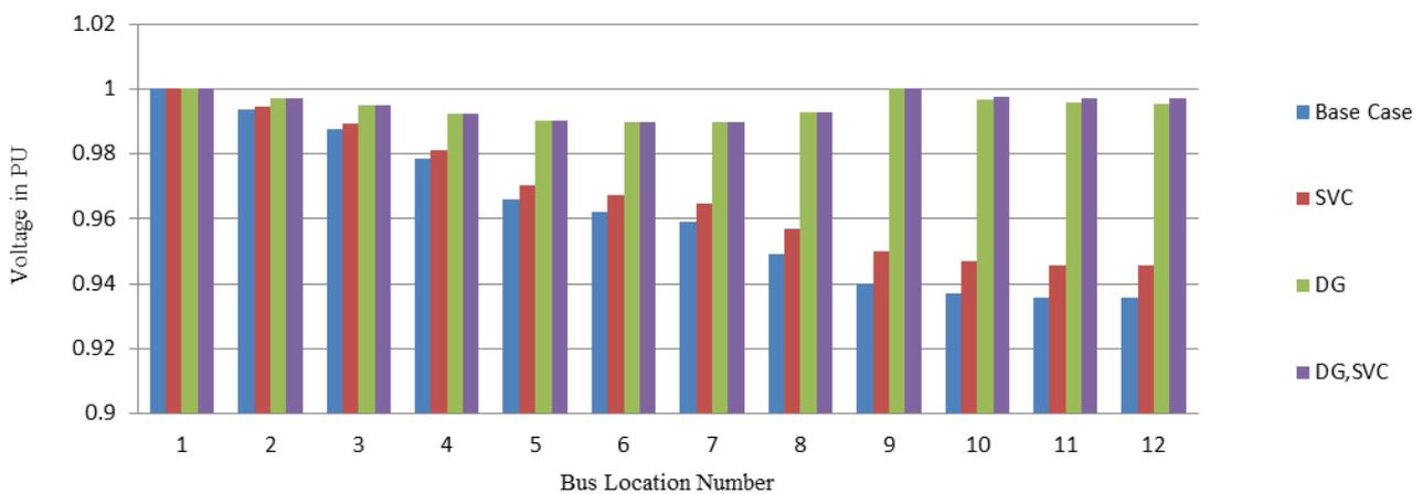
Fig. 5. Voltage profile of 12 Bus system
