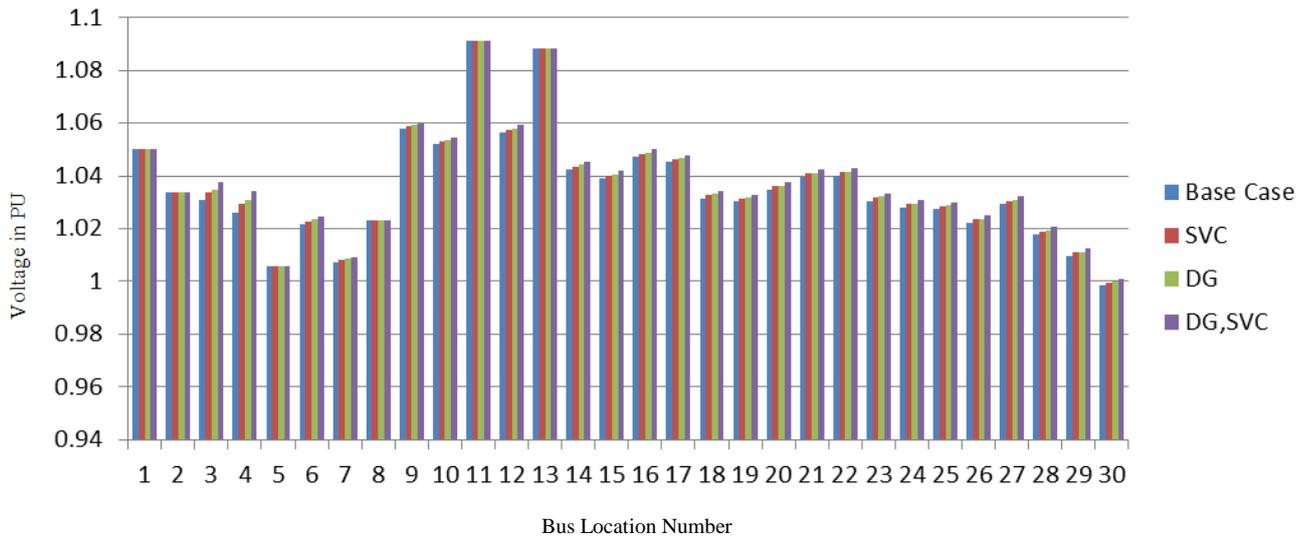
Fig. 4. Voltage profile of 30 Bus system
