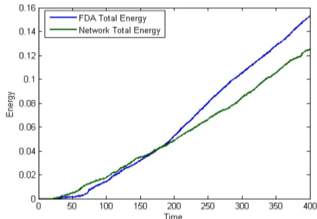
Fig. 8. Comparing the total energy in normal WSN and FDA WSN
