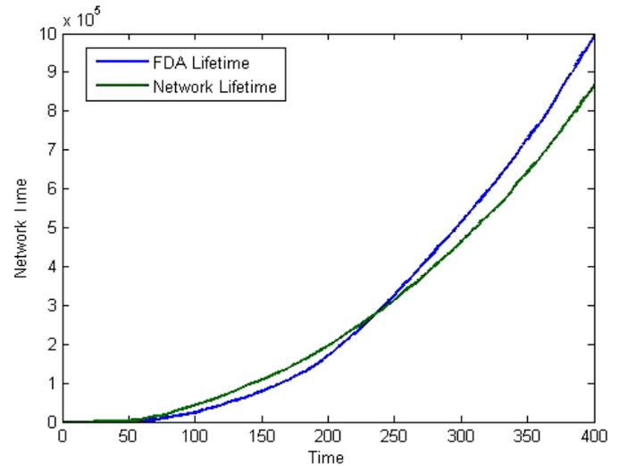
Fig. 12. Comparing the network life time between normal WSN and FDA WSN
