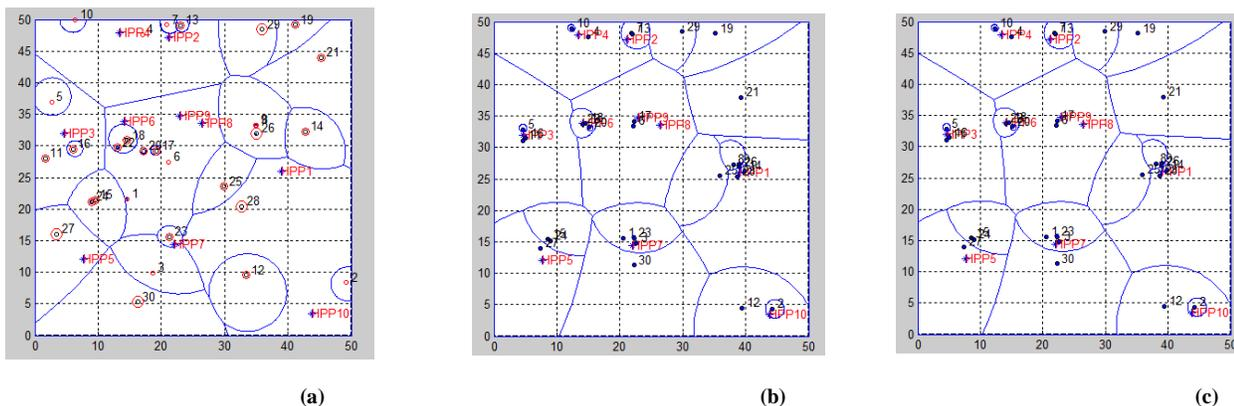
Fig 3 Snapshots of (a) Initial Coverage (b) Intermediate Coverage and (c) Final Coverage of 30 sensors deployed in the target area where Euclidean distance alone is considered
