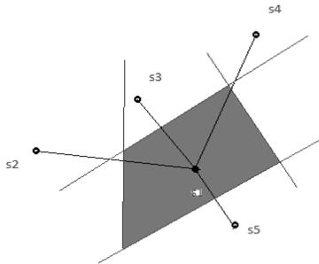
Fig 1. Voronoi Region for sensor node  $S_1$  with  $S_2, S_3, S_4, S_5$  as neighbors
