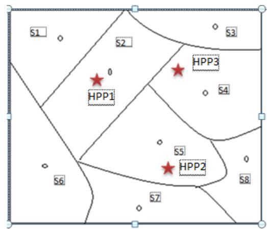
Fig 2. MW-Voronoi Regions with 8 sensors and 3 HPP
