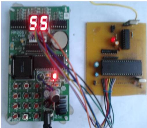
**Fig. 11 Robotic car Transmitter circuit**
