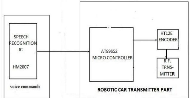
**Fig. 7 Robotic car transmission part**
