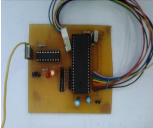
**Fig. 10 RF Transmitter circuit**
