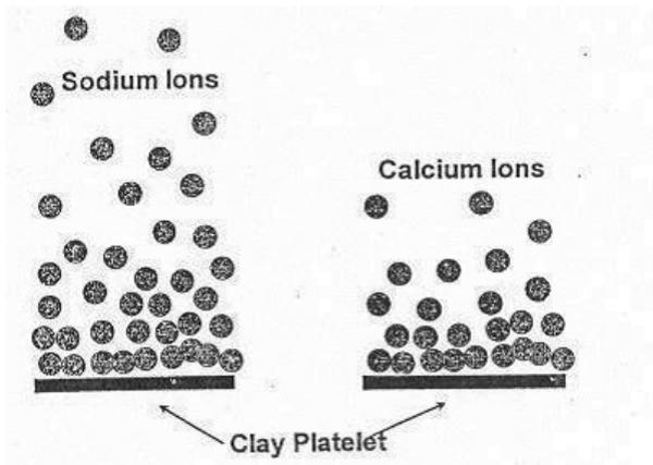
**Figure 2: Behavior of sodium and calcium ions attached to a clay platelet. (Source: Hanson et al., 1999)**
