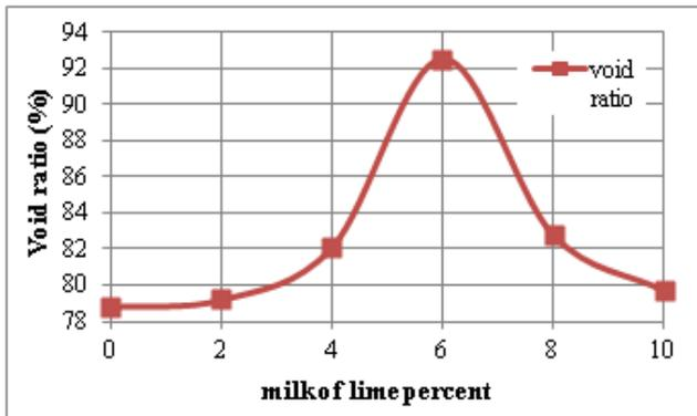
**Figure 7: Milk of lime effect on void ratio**
