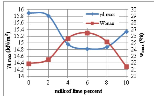
Figure 5: Milk of lime effect on the optimum Proctor
