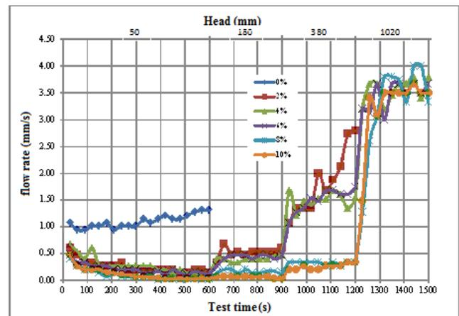
**Figure 9: Flow rate vs time in the pinhole test**
