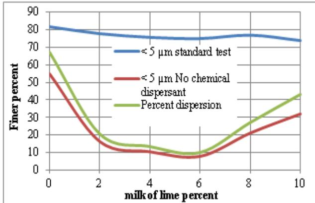
**Figure 1: Percent dispersion as determined from the double hydrometer test**
