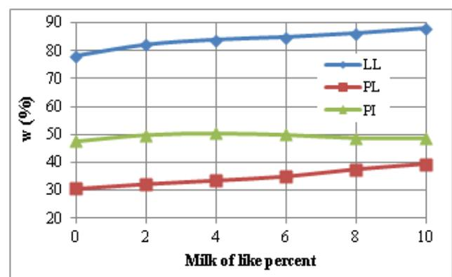
Figure 6: Milk of lime effect on Atterberg limits
