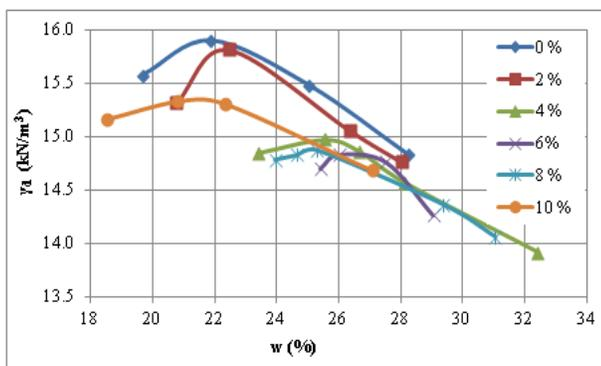
Figure 4: Milk of lime effect on the Proctor curve
