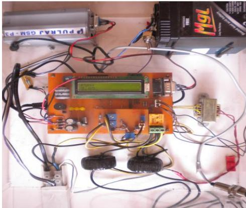
**Fig:-5 Designed energy meter**
