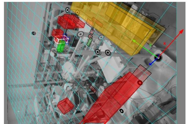
**FIGURE 4 VIEW OF SAFETY CAMERA AND DEFINED DETECTION ZONES**
