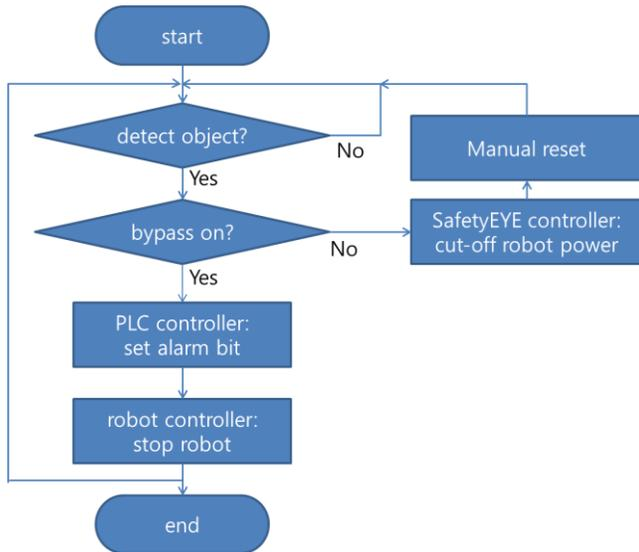
**FIGURE 5 FLOW OF SAFETY CONTROL LOGIC**
