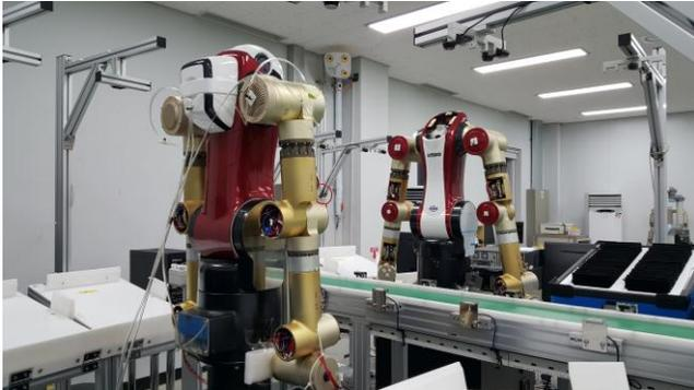
**FIGURE 2 CELL PRODUCTION LINE WITH TWO DUAL-ARM ROBOTS**
