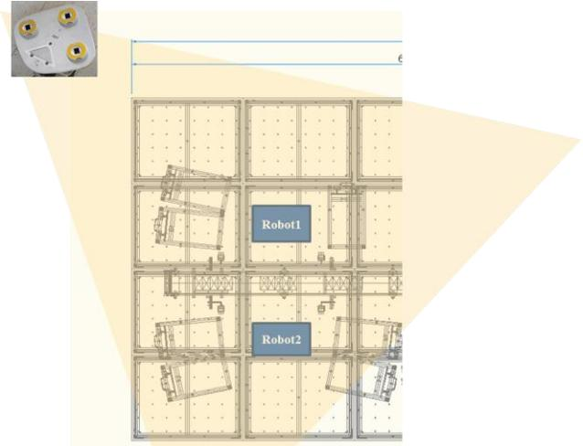
**FIGURE 6 POSITION OF SAFETY CAMERA IN DEMO LINE**
