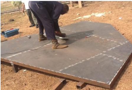
**Fig. 3: Forming the base of the Mould**
