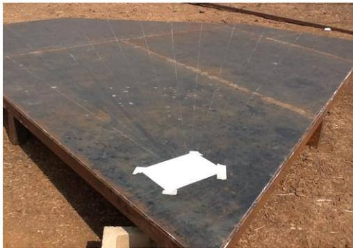
**Fig. 2: Forming the base of the Mould using pencil and marker**
