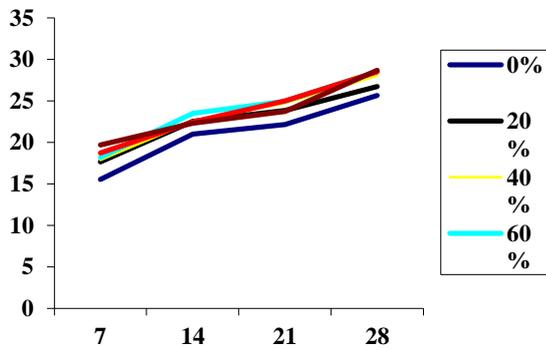
**Fig.1. Compressive Strength of varied percentages of foundry sand concrete with varied curing day**
