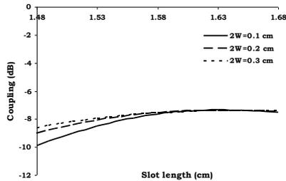
**Fig.5** Variation of coupling with slot inclination  $\theta_s = 40^\circ$
