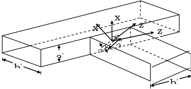
**Fig.1 Inclined slot coupled waveguide shunt Tee- non-standard waveguide**
