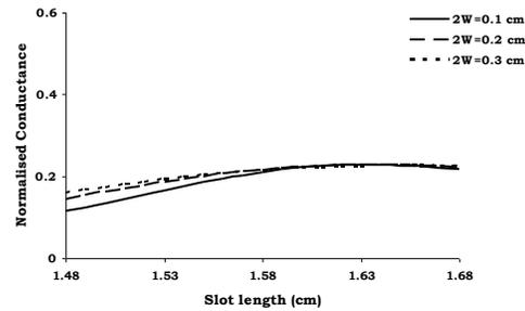
Fig.3 Variation of normalized conductance with slot inclination  $\theta_s = 40^\circ$
