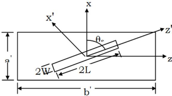
**Fig. 2 Inclined slot in the narrow wall**
