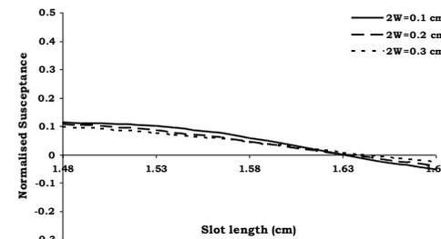
Fig.4 Variation of normalized susceptance with slot inclination  $\theta_s = 40^\circ$
