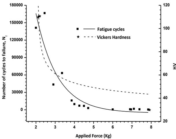
**Fig. 9** Variation of Number of Cycles and Vickers Hardness with Applied Force for AA6063 as received
