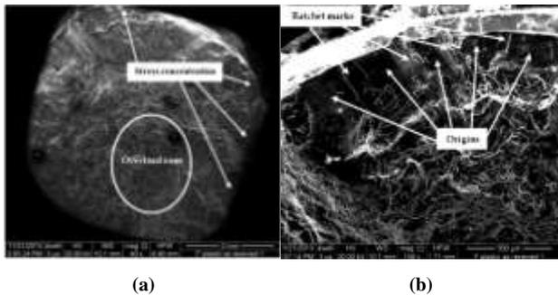
**Fig. 13: SEM Pictures after the LCF test at the plastic zone at: (a) 40x magnification ,(b) 150x magnification**
