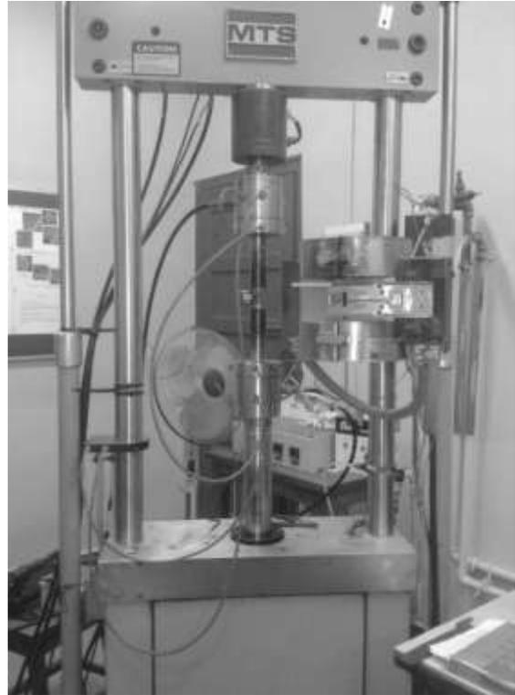
**Fig. 2 Tensile Testing Machine**
