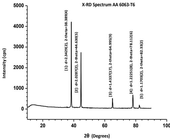
**Fig. 6 X-RD Pattern for as received AA6063-T6 alloy at room temperature**
