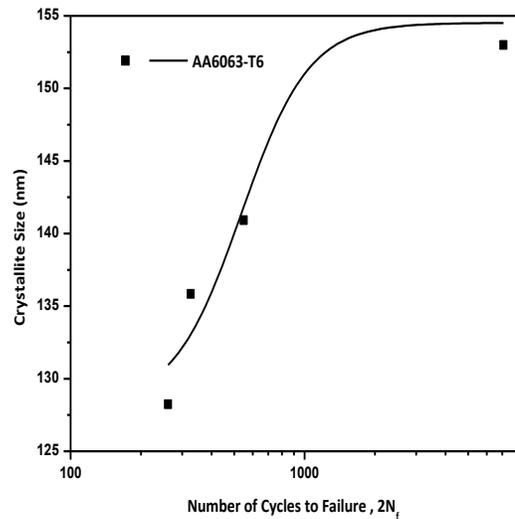
Fig. 8 Crystallite Size with the Number of Cycles to Failure
