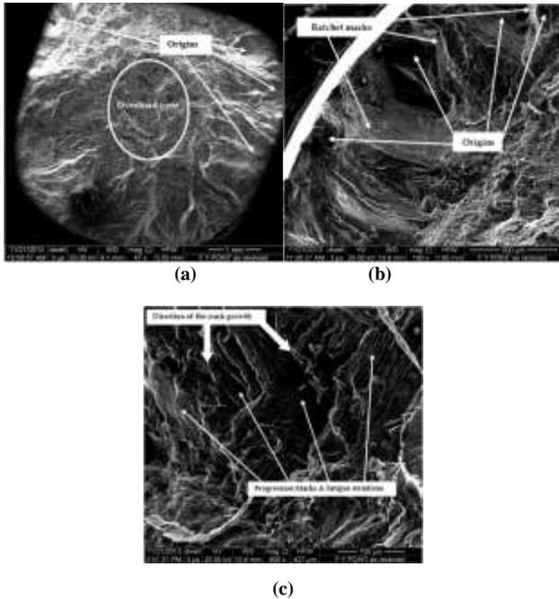
**Fig. 12: SEM Pictures after the LCF test at the Yield point at: (a) 47x magnification, (b) 160x magnification, (c) 600x magnification**
