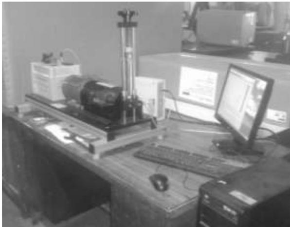
**Fig. 5 Cantilever Fatigue Testing Machine**
