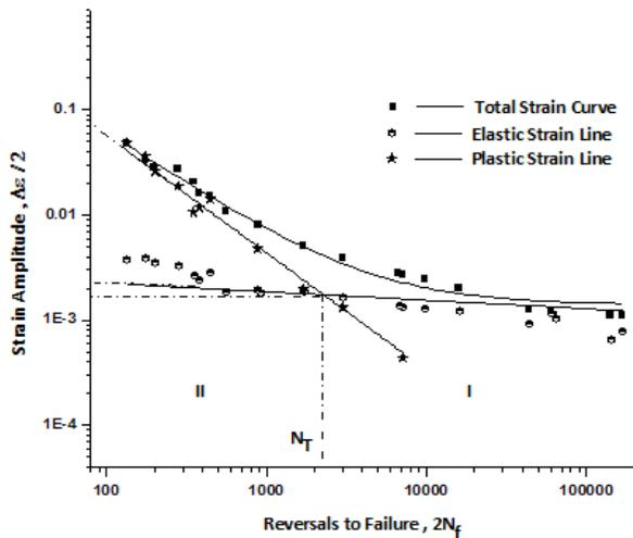
Fig. 7: Strain life Curve for as received AA6063-T6 alloy at Room Temperature
