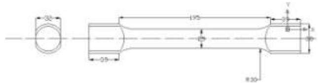
**Fig. 3 Torsion Test Specimen**
