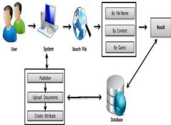
**Figure-4: System Architecture of facilitating document Annotation using content and querying value.**
