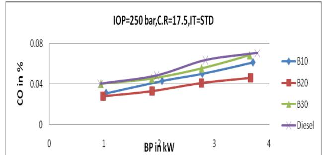
**Fig 6.8: Carbon monoxide v/s Brake power**
