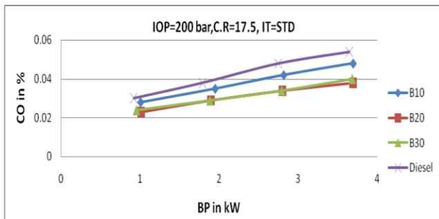
**Fig 6.7: Carbon monoxide v/s Brake power**
