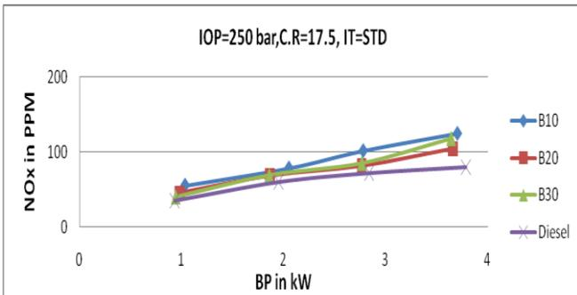
**Fig 6.17: Nitrogen Oxide v/s Brake Power**
