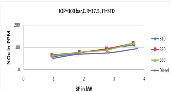
**Fig 6.18: Nitrogen Oxide v/s Brake Power**
