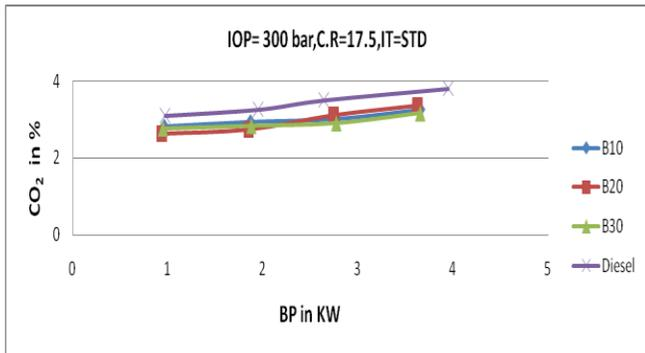
**Fig 6.12: Carbon Dioxide v/s Brake Power**
