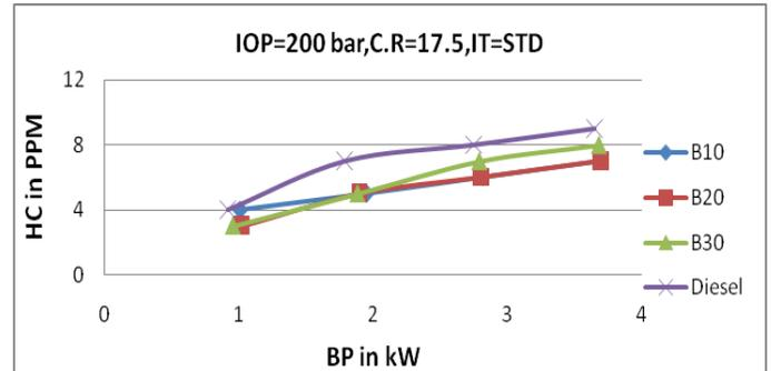
**Fig 6.13: Hydro Carbon v/s Brake Power**
