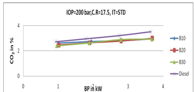
**Fig 6.10: Carbon Dioxide v/s Brake Power**
