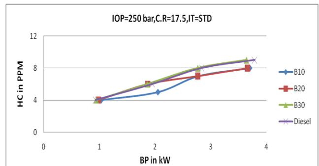
**Fig 6.14: Hydro Carbon v/s Brake Power**
