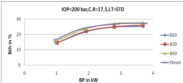
**Fig 6.1 Brake thermal efficiency v/s Brake power**
