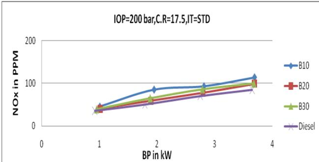
**Fig 6.16: Nitrogen Oxide v/s Brake Power**
