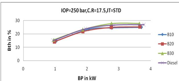
**Figure 6.2 Brake thermal efficiency v/s Brake power**
