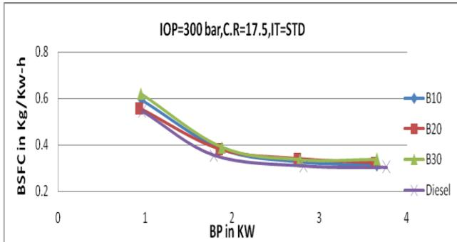
**Fig 6.6: Brake specific fuel consumption v/s Brake power**
