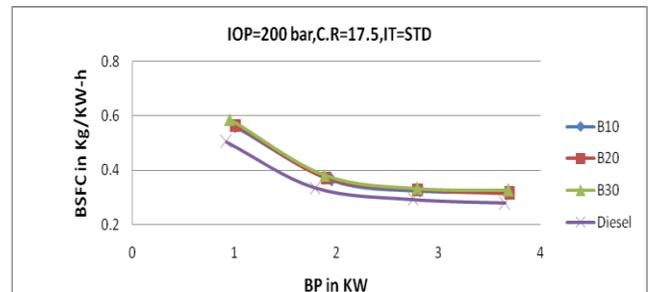
**Fig 6.4: Brake specific fuel consumption v/s Brake power**
