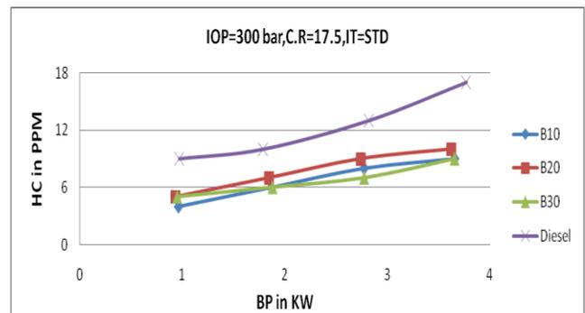
**Fig 6.15: Hydro Carbon v/s Brake Power**
