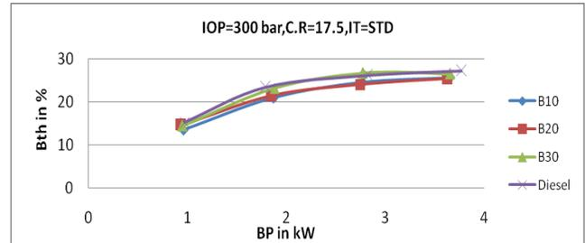
**Fig 6.3 Brake thermal efficiency v/s Brake power**
