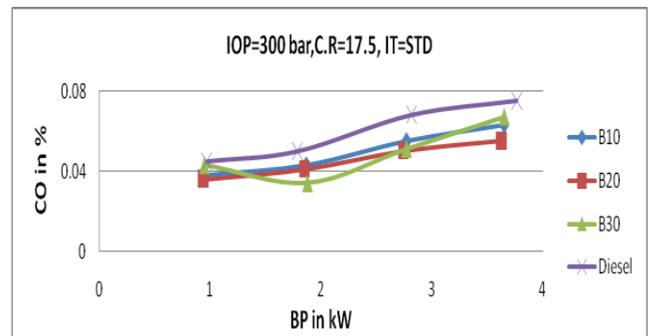
**Fig 6.9: Carbon monoxide v/s Brake power**
