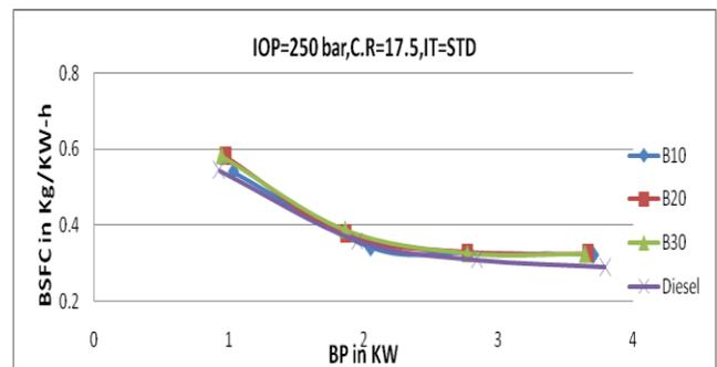
**Fig 6.5: Brake specific fuel consumption v/s Brake power**
