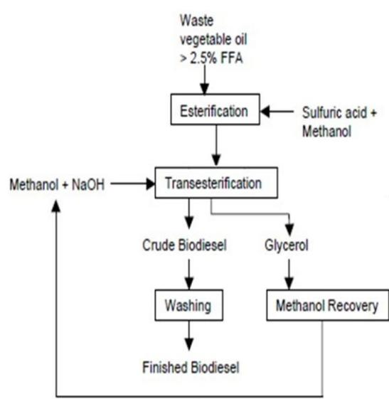
**Fig 1 Steps for Production of Biodiesel from Vegetable Oil**
