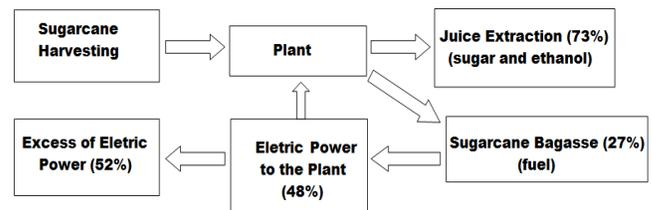
**Fig. 2. General Cogeneration scheme using sugarcane bagasse. Source: Self elaboration**
