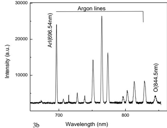
**Fig.3: Optical emission spectra of atmospheric pressure plasma jet at jet length of 3.5cm**
