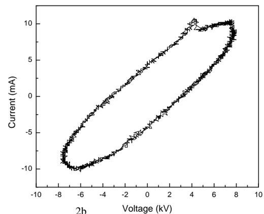
**Fig.2: Current voltage signal of APPJ and Lissajous figure**
