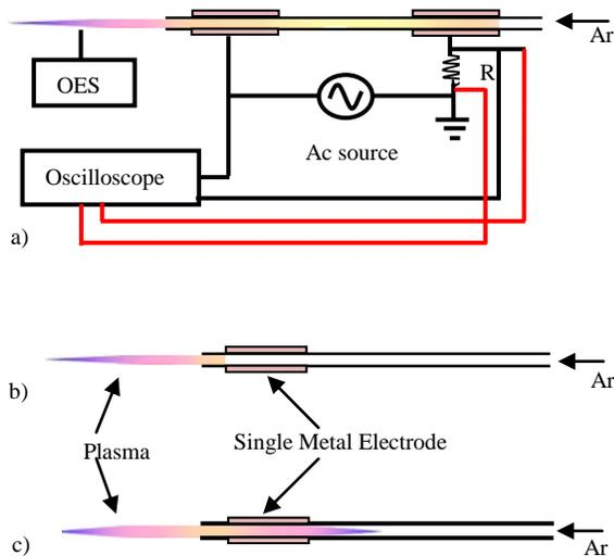
**Fig.1: Schematic diagram of experimental setup for generation of atmospheric pressure argon plasma jet. a) plasma jet with double electrode b) plasma jet downstream with single electrode c) plasma jet downstream and upstream with single electrode**
