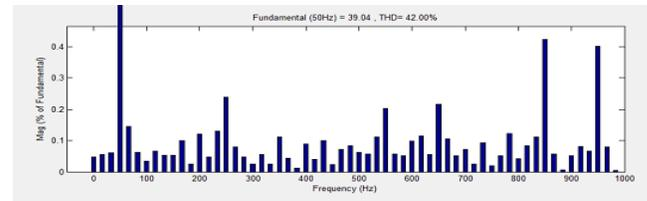
**Figure 6. THD of 3-level Diode Clamped MLI**
