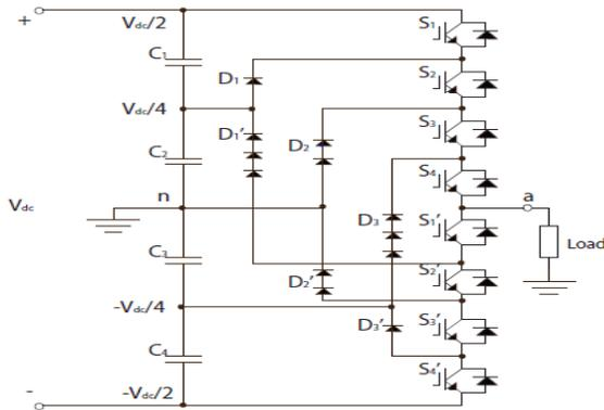
**Fig.3. 5-level Diode Clamped Inverter**
