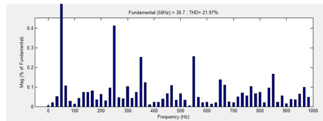
**Fig.7. THD of 5-level Diode Clamped**
