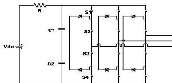
**Fig. 2. 3-Phase,3-level Diode Clamped Inverter**
