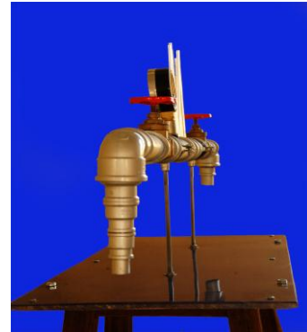
Plate IV: 3D view of fabricated Venturi meter .
