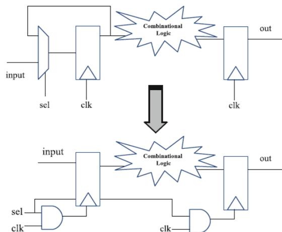
**Fig.2: In pipelined styles, the effectiveness of clock gating may be increased. If the inputs to a pipeline stage stay a similar, then the clock to the later stages may also be frozen**
