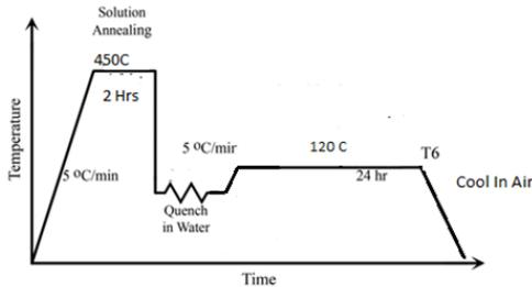
**Figure 1: Schematic of conventional heat treatment cycle (single step ageing).**
