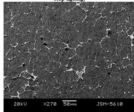
**Figure 5d: Modified T6 Heat treated (Double step ageing)**
