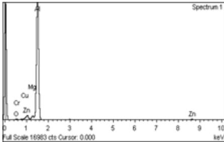
**Figure 4: X-ray spectrum of as cast 7075 alloy.**
