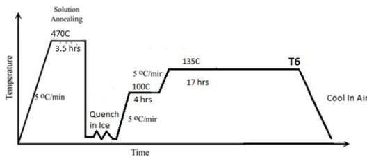
**Figure 2: Schematic of modified heat treatment cycle (dual step ageing).**
