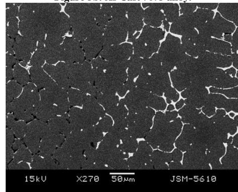
**Figure 5c: Conventional T6 Heat treated (Single step ageing)**
