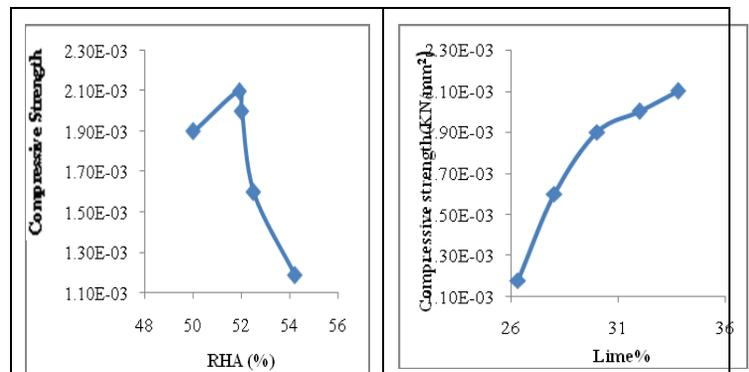
**Fig. III: Compressive Strength vs RHA and Lime**
