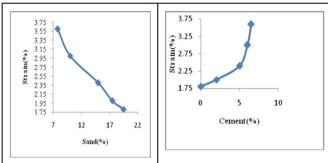
**Fig. VI: Strain vs Sand and Cement**
