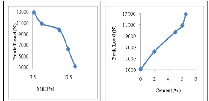
**Fig. VIII: Peak Load vs Sand and Cement**
