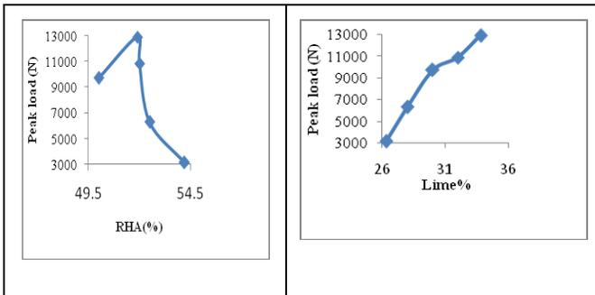
**Fig. VII: Peak Load vs RHA and Lime**
