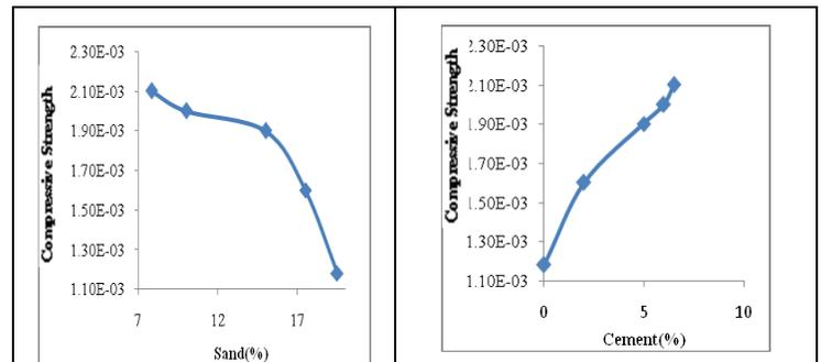
**Fig. IV: Compressive Strength vs Sand and Cement**
