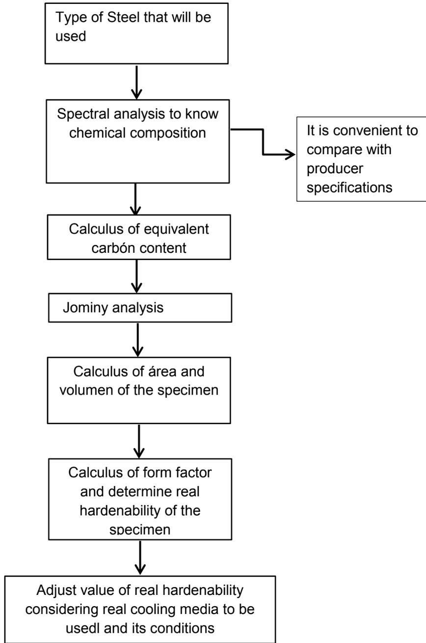
FIG. 2 Algorithm for the correct calculation of the hardenability of a piece.
