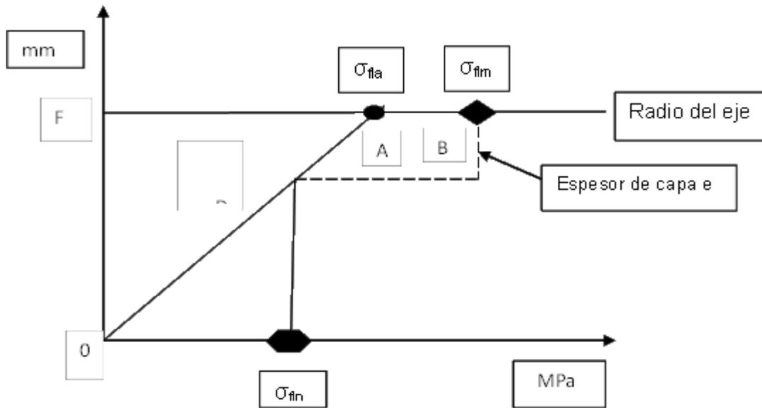
**Fig.3 Schematic for calculating the layer thickness depending on the efforts of acting bending.**
