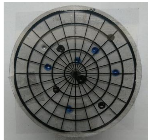
b) with indentation (Blue indents are for BHN and Black for Rockwell B scale.)
