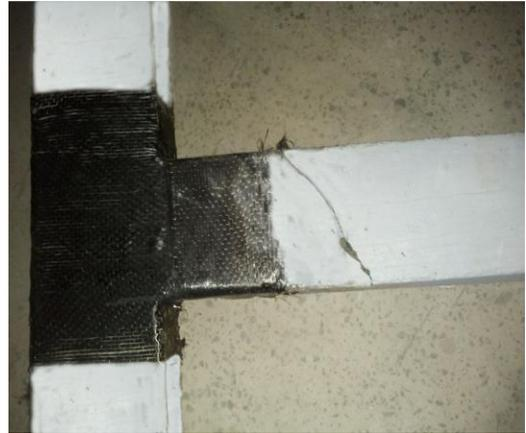
**Fig. 9. Crack Pattern of BCJ CF-01**
