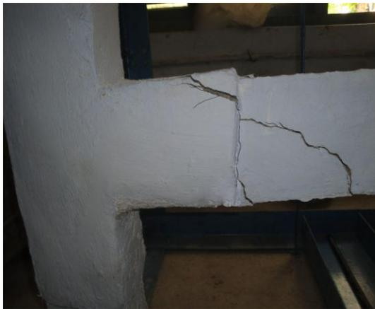
**Fig. 8. Crack Pattern of BCJ FC**
