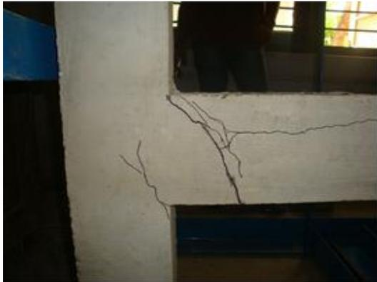
**Fig. 7. Crack Pattern of BCJ**
