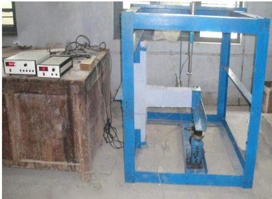
Fig. 4. Test setup with beam column joint specimen
