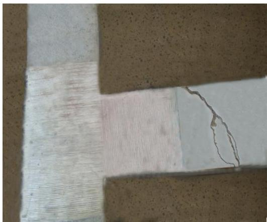
**Fig. 12. Crack Pattern of BCJ GF-02**
