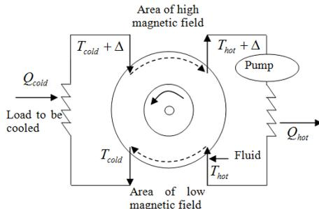
Fig. Schematic representation of the Steyert's magnetic system.
