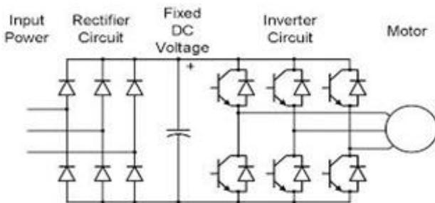
**Fig.3 VFD schematic diagram[13]**
