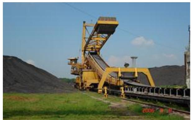
Fig.1 photograph of stacker/reclaimer [13]
