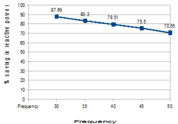
Fig.7 graph between freq. & % saving in reactive power
