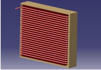
From upper tank water enters copper tubes and by gravity, it flows through those tubes.
