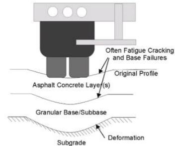
**Figure 1 Structural rutting [7]**
