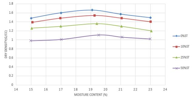
**Fig 3.3: Compaction Behaviour of Clay and Clay –Shredded Tyres Mixture of Size 30mm**
