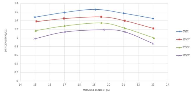
**Fig 3.4: Compaction Behaviour of Clay and Clay –Shredded Tyres Mixture of Size 50mm**
