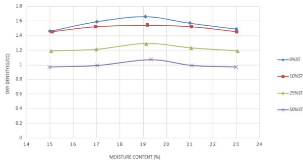
**Fig 3.2: Compaction Behaviour of Clay and Clay –Shredded Tyres Mixture of Size 10mm**
