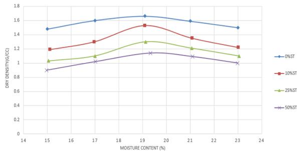
**Fig 3.1: Compaction Behaviour of Clay and Clay –Shredded Tyres Mixture of Size 5mm**
