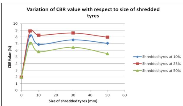
**Fig 4.1** Variation of CBR Values of shredded tyres with respect to size of shredded tyres.
