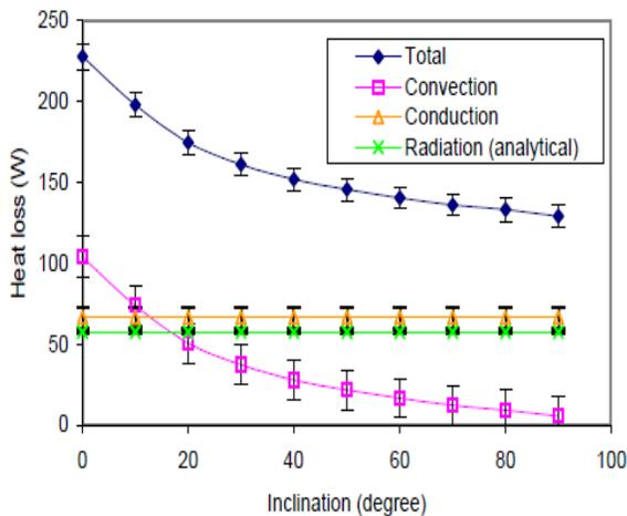
**Fig. 3 Experimental heat loss for a cavity temperature of 450°C [49].**
