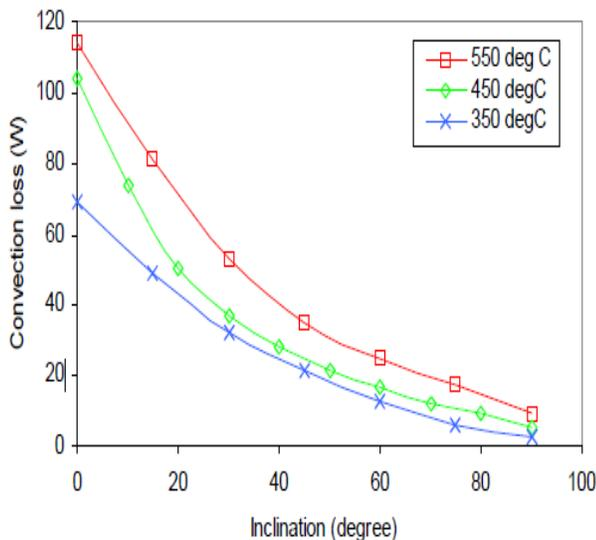
**Fig. 4 Convection loss at various cavity temperatures [49].**
