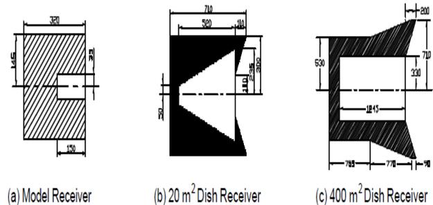
**Fig. 5 Three Receiver Systems and Cross Sectional Diagram of All Three Receiver Models [51].**
