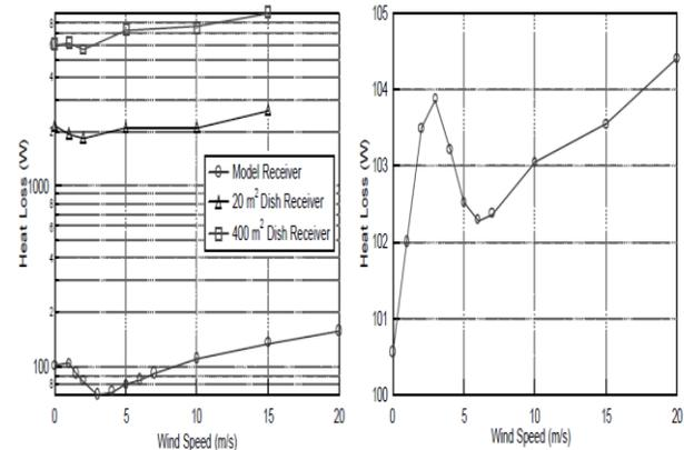
**Fig. 6 The Relationship between Wind Speed and Heat Loss for Model Receiver with Wind Parallel to the Aperture Plane [51].**
