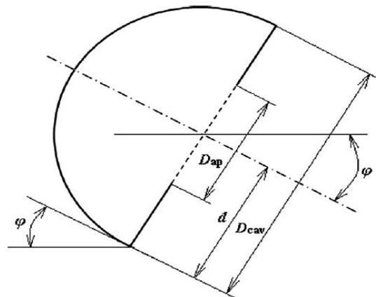
**Fig. 2 Main features of tilted open rectangular or cylindrical cavity [16].**
