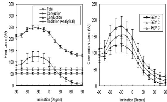
**Fig.9** Experimental heat loss with Convection heat loss from  $T_c=445^\circ$  & a fully open cavity [39]
