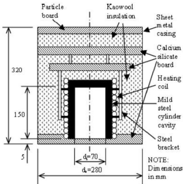
**Fig. 8** Cross section sketch of model receiver [39].
