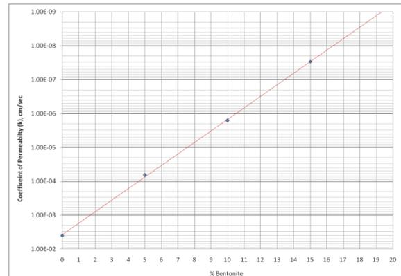
**FIGURE V VARIATION OF COEFFICIENT OF PERMEABILITY WITH PERCENTAGE OF BENTONITE**
