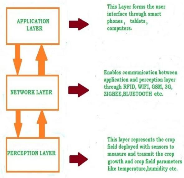
**Fig 1 : Three layer structure of IoT.**
