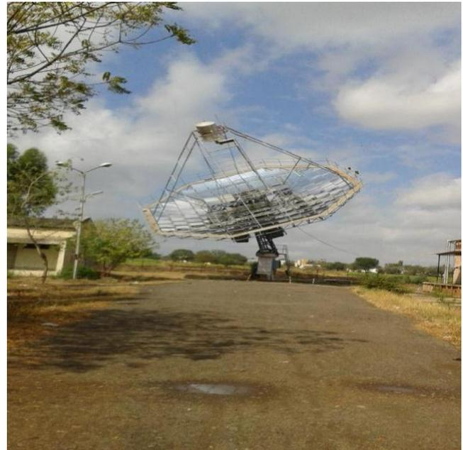
Method to utilise concentrated solar energy have been develop to achieve higher operating temperature and efficiency in solar thermal system. the technology used to achieve the higher working temperature is concentrating solar power in cavity shape receiver. the cavity receiver are positioned at the focus of the dish, allowing the collection of concentrated solar rays.
