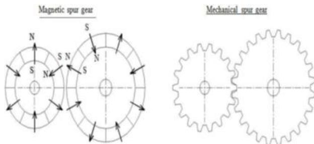
**Figure 4: Magnetic spur gear with magnets and mechanical spur gear**
