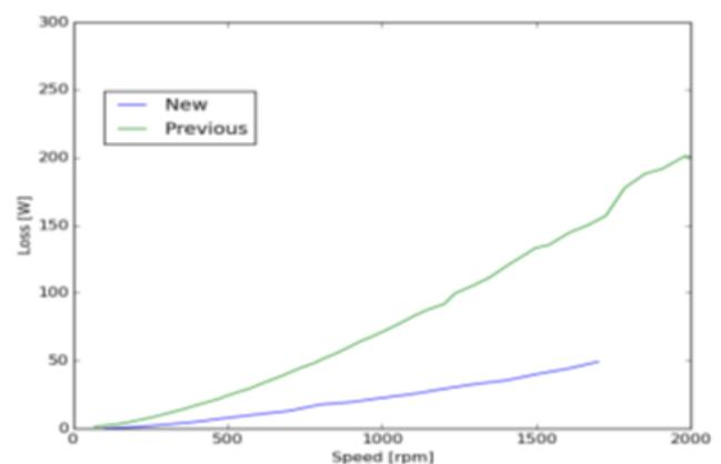
**Figure6: Comparison of no-load loss between the previous and the improved magnetic gears.**
