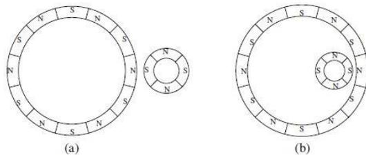
**Figure 3 External & Internal Meshing of gears**
