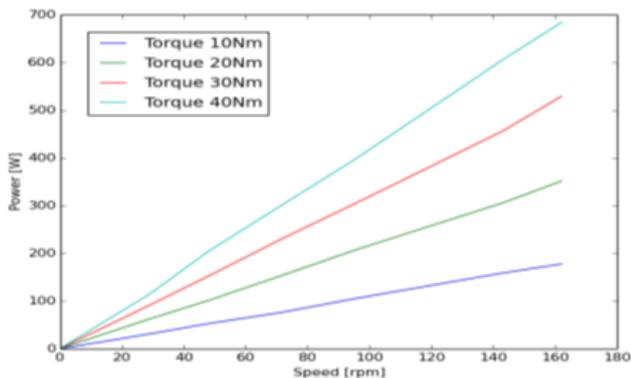
**Figure 7: The output power of the magnetic gear as a function of speed for different loads (on low speed side)**
