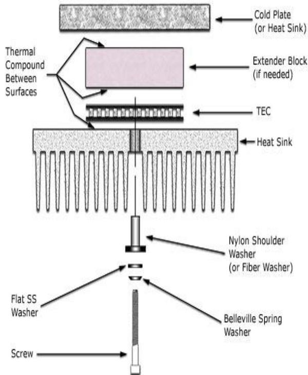
**Fig.5. Assembly of components**
