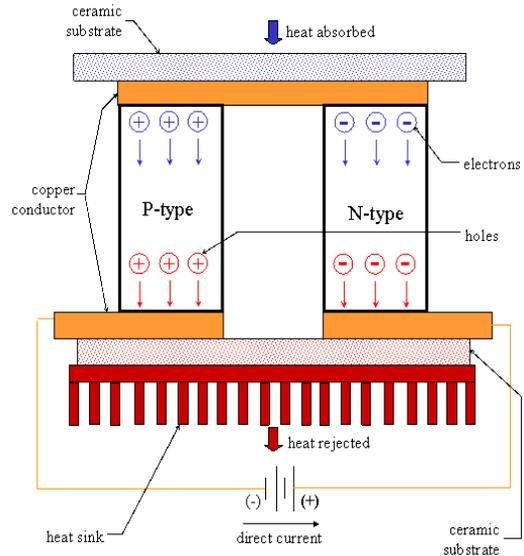
**Fig .3. Thermoelectric cooler**
