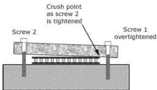
**Fig 6. Crushing due to over tight**
