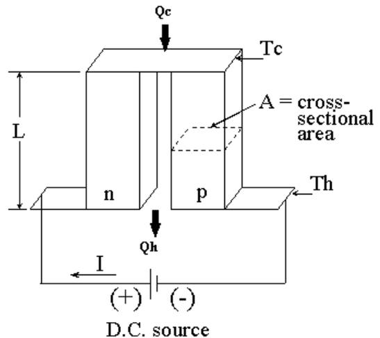
**Fig .4. Notations of Thermoelectric Module**
