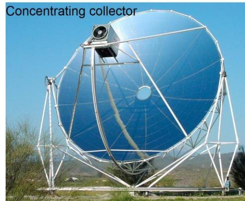
**Fig.3 concentrating collector<sup>[2]</sup>**
