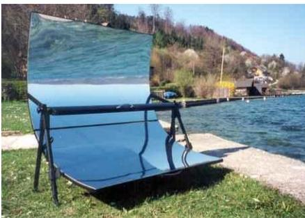
**Fig.2: cylindrical solar collector**
