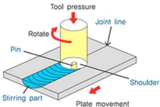
**Fig:2 Solid state welding**
