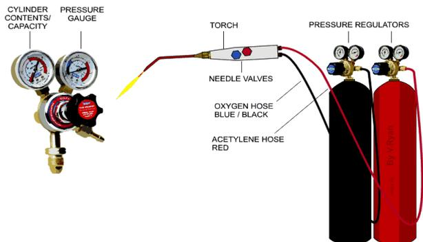
**Fig:1 Oxy-acetylene gas welding.**
