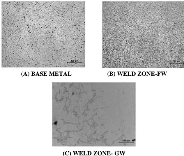
**Fig:3 Different Zones Of Welded Joints**
