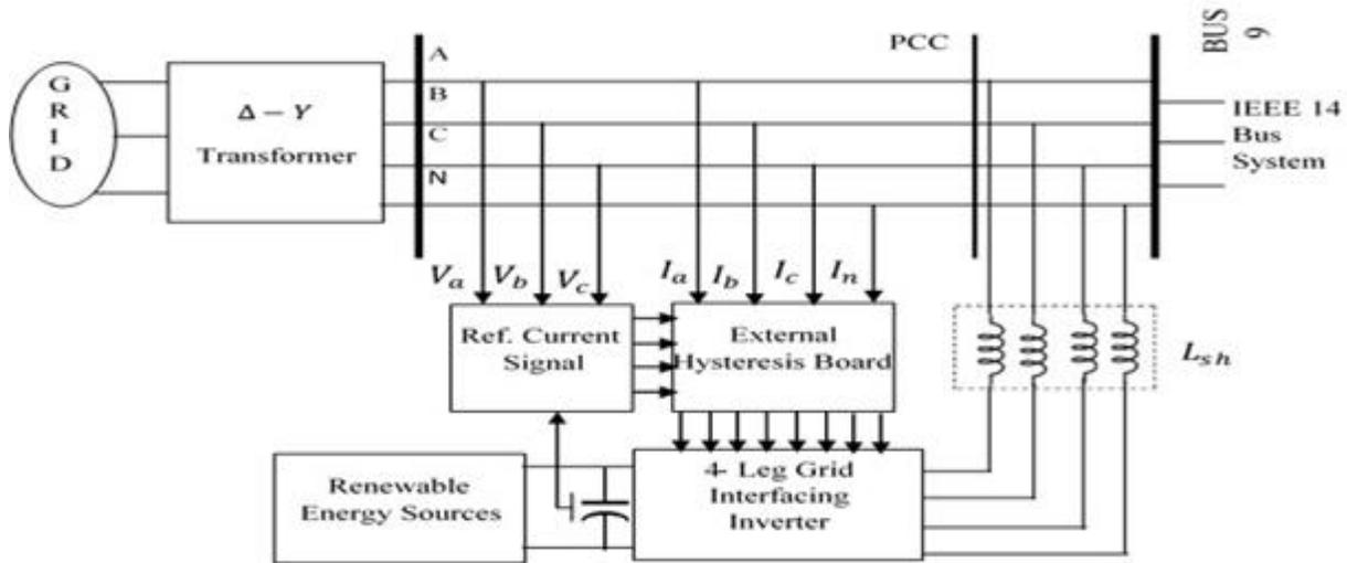
**Fig.1 Schematic of Renewable Based Distributed Generation System [8],[12]**
