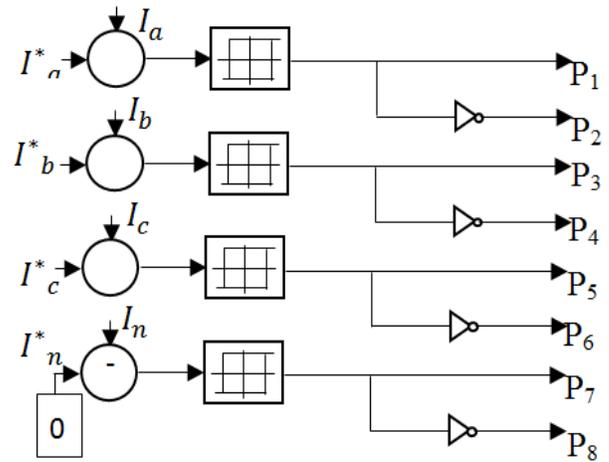
**Fig.4 Gate Pulse Generation**
