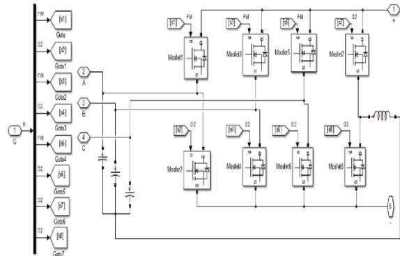
**Fig.5 SIMULINK Model of 3-Phase 4-Leg Grid Interfacing Inverter.**
