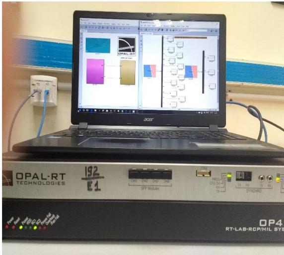
**Fig. 10 OPAL-RT Model Interfaced with OP4510**
