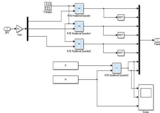
**Fig.6 SIMULINK Model of PWM Pulse**
