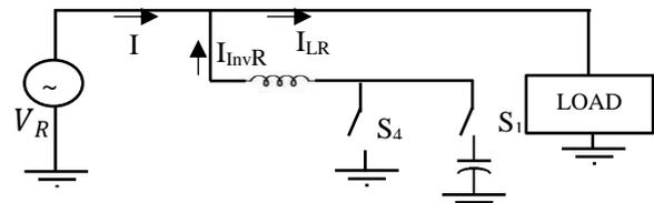
**Fig.3 Single Phase Equivalent Circuit of the System and VSI**
