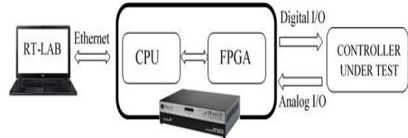
**Fig.2 Schematic of OPAL-RT Implementation**
